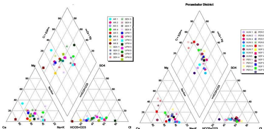
**Fig. 1. Groundwater Samples from Ariyalur (on left) and Perambalur (on right) Districts Plotted Piper-Trilinear Diagram**
