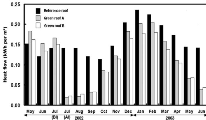
**Fig. 3 - Comparison of the average daily heat flow through the green roofs and reference (conventional) roof over two years.**
