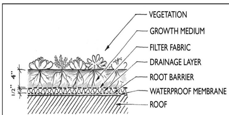
**Fig. 2 – Cross-section of extensive Green roof prototype**
