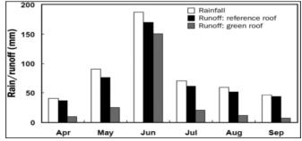
Fig. 4. Storm-water runoff retention in a green-roof test plot in Ottawa, Ontario, Canada, in 2002.
