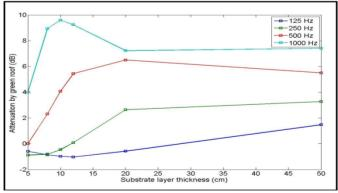
Fig. 5: Attenuation of Noise by green roof Source - http://www.acoustics.org/press/155th/renterghem.html
