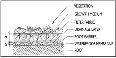
**Fig. 2 – Cross-section of extensive Green roof prototype** (Source - *amalthea.kevio.gr/wp.../Tapping-the-potential-of-urban-rooftops.pdf*)
